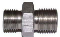
BT-1522 1/4" BSP male with 60° female cone to 9/16" UNF male adapter
