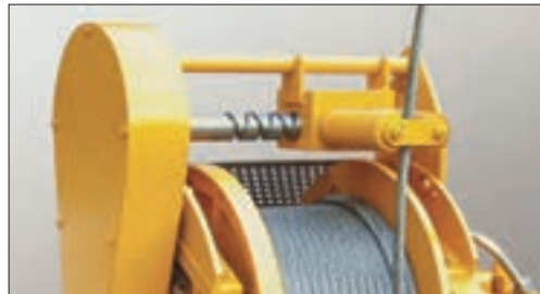
Spooling device on LS5000R
