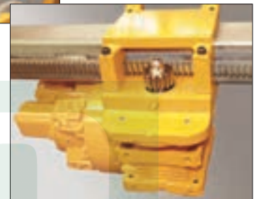
Precision cut rack & pinion drive assembly
